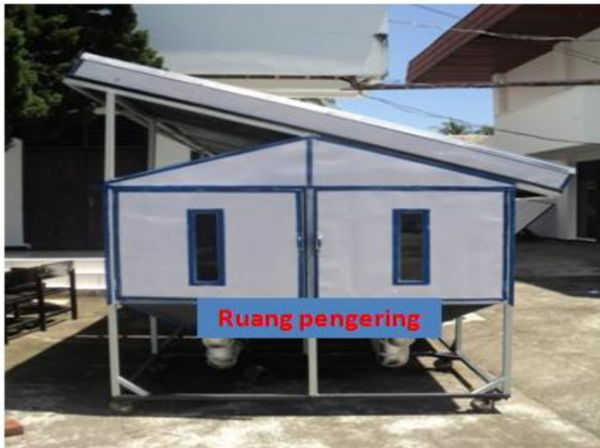
Gambar.4 Photo ruang pengering
